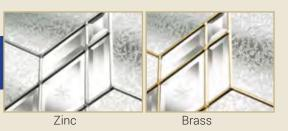
Our Platinum Clarity, Kara and Simplicity triple glazed style designs are constructed using hand-cut bevels and beautifully textured glass pieces, which are assembled using traditional stained glass methods into zinc or brass cames. The decorative glass is then encapsulated between two pieces of clear safety glass to give excellent thermal and sound insulation with the added benefit of an easy to clean, smooth surface.
